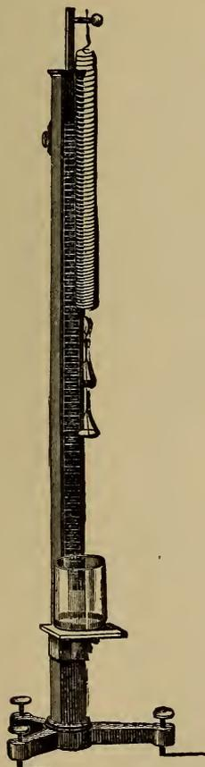
Fig. 82. PROF. JOLLY'S APPARATUS FOR DETERMINING THE SPECIFIC GRAVITY OF MINERALS.
